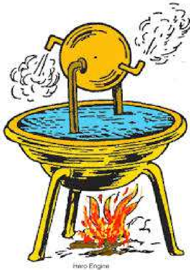
Figure 10.8: A jet-driven steam engine invented by Hero of Alexandria in the 1st century A.D..
