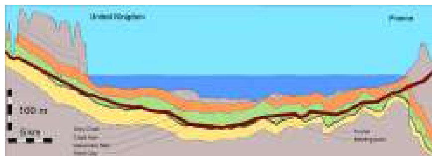
Figure 5.28: Geological profile along the tunnel as constructed. For most of its length the tunnel bores through a chalk marl stratum.
