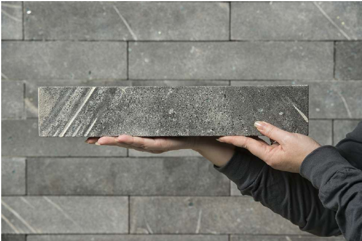
Figure 2.21: BioMason uses bacteria to grow cement bricks which it says can sequester carbon. Credit: bioMASON, Inc..
